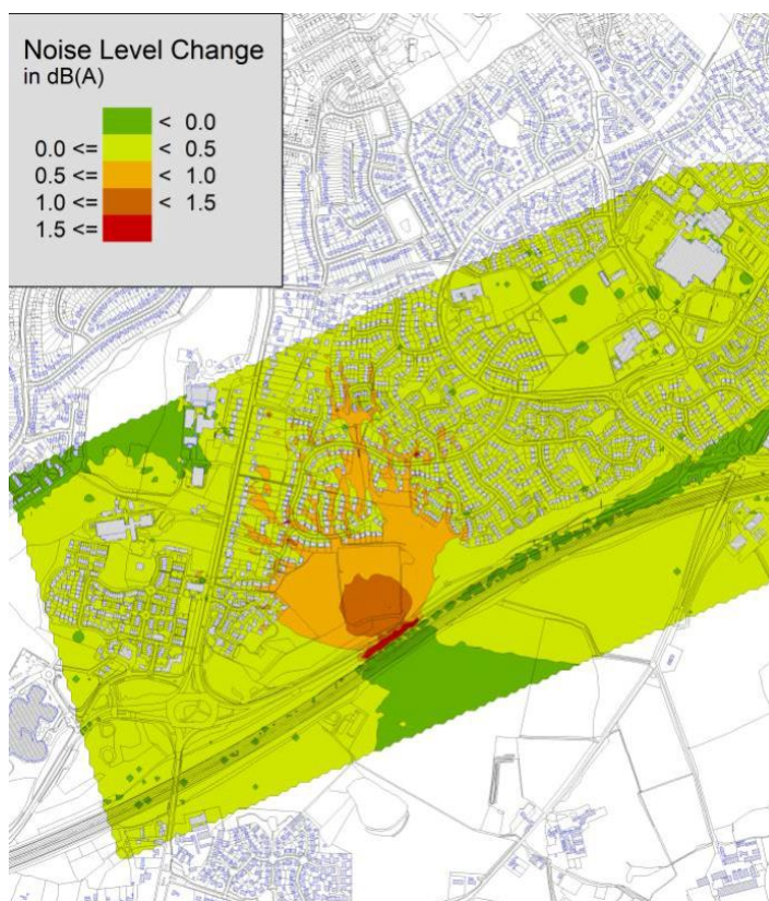
Figure 1 Change in noise levels due to removal of 150 metres from barrier (west end)
